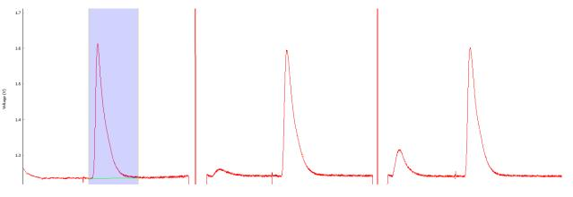
Figure 1: Raw ACOMP detector signal
