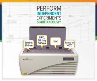
ARGEN is a powerful tool for biopharmaceutical and polymer scientists. With 16 sample cells, each independently capable of precise control of thermal, chemical and mechanical stress, and via static light scattering, ARGEN measures the pharmaceutical stability of therapeutic proteins and peptides and the quality of natural and synthetic polymers.
